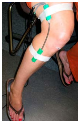
Figure 20.6 Attach a goniometer (SS20L) to the outside of the knee.
